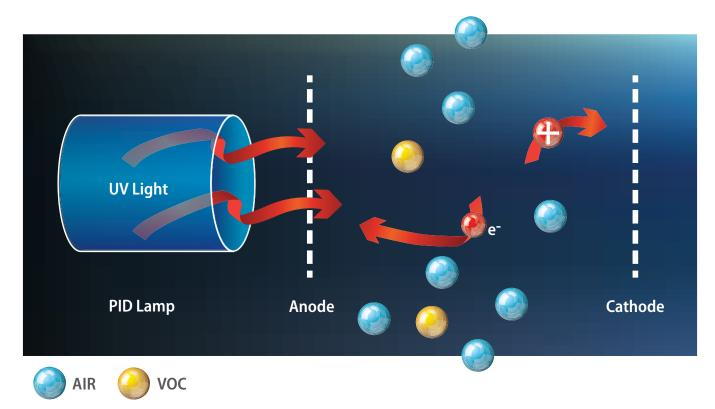
Most substances can be ionized, some more easily than others. The ability of a substance to be ionized is measured as ionization potential (IP) using an electron volt (eV) energy scale. This scale generally runs from a value of 7 to a value of approximately 16. Substances with an eV rating of 7 are very easy to ionize; substances with an eV rating of between 12 and 16 are extremely difficult to ionize. IP ratings of some common substances include:
